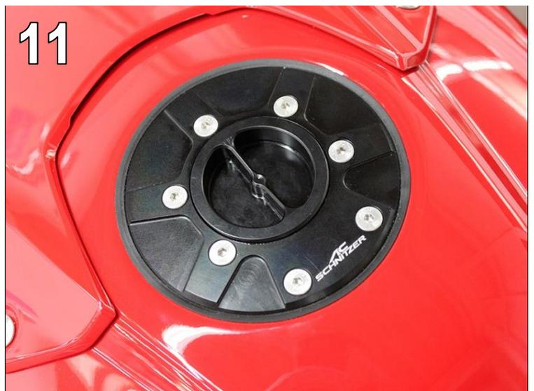
Check the fastening screws for tightness.
