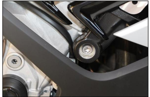
Insert the enclosed cap screws with washers through the base plate / holder, insert anti-rotation devices in the groove and fasten them so that they can still be moved.
