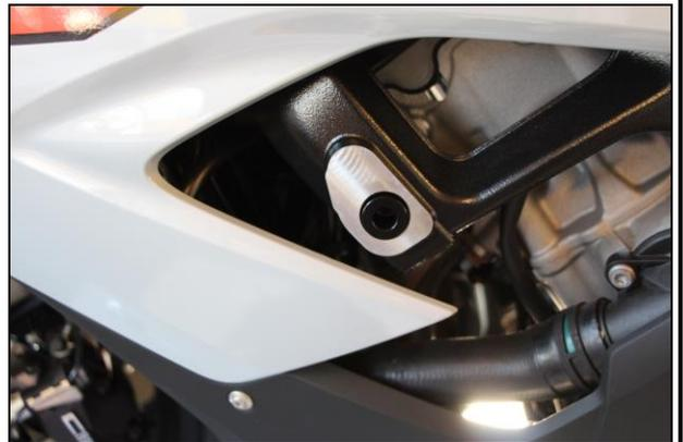
Attach the base plate / holder to the vehicle frame.
