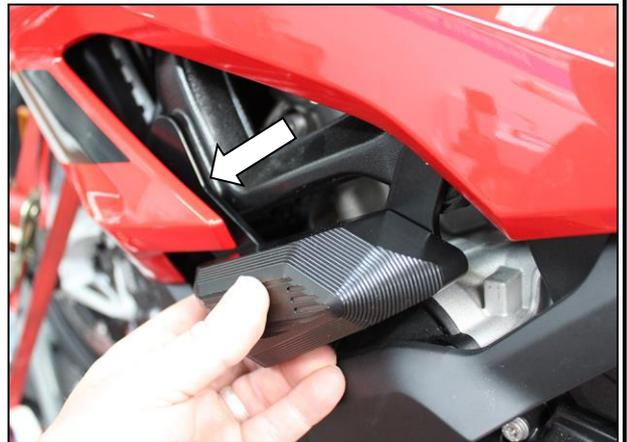
Insert the base plate / holder at the rear motor mounting point in the bore and at the front mounting point with the washer and screw on the frame fixing screws -60 Nm.
