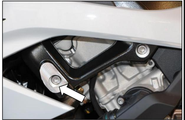
Insert the enclosed spacer sleeves into the frame.
