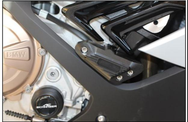
Clean the recess in the crash pad and insert the sticker and press it firmly into place.
