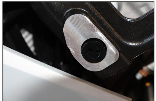
Place the base plate / holder between the frame with the with the supplied washer and screw.
