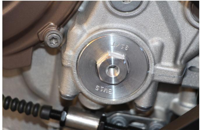
Fit the motor pad with the enclosed screw and washer.
